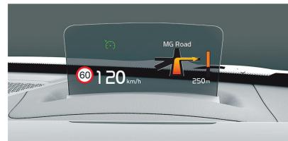
HUD makes driving safer by minimizing the movement of driver's line of sight
