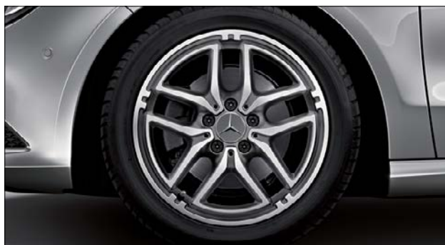
5-twin-spoke wheel Finish: Himalaya Grey, high-shine Wheel 7.5 J x 17 ET 52.5 | Tyre 225/45/R17 A24640115027X21
