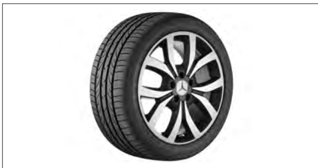
5-twin-spoke wheel - red rim flange, black Wheel: 7.5 J x 18 ET 52 Tyre: 225/40/R18
