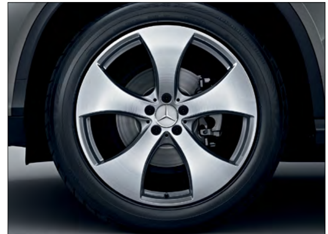
5-spoke light-alloy wheels, painted himalayas grey with a high-sheen finish, with 275/45 R21 front and 315/40 R21 rear tyres
